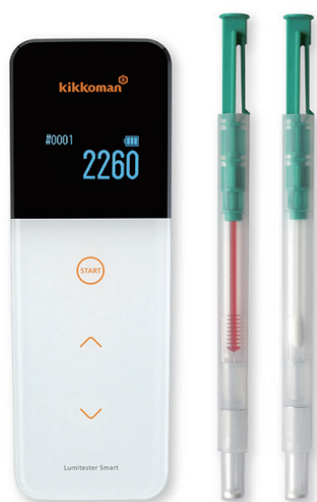
Measuring instrument 'Lumitester Smart' and measurement reagent 'LuciPac A3'
