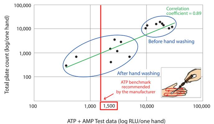
Figure 7: Correlation between an ATP Test and a microorganism test before and after hand washing
