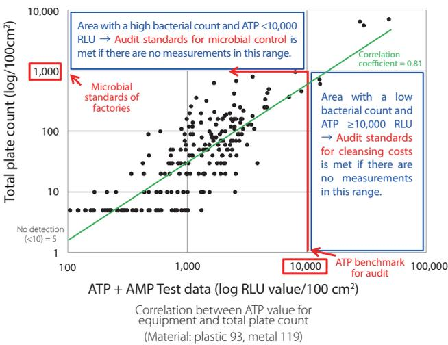
**Figure 3:** Correlation between an ATP Test and a microorganism test in a fresh meat processing factory
