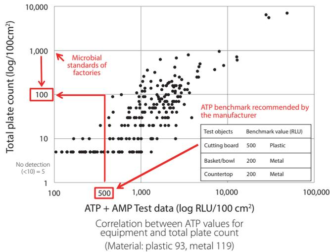
Figure 4: Microbial standard of 100/100 cm<sup>2</sup> with 500 RLU used as the benchmark
