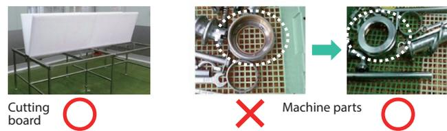
**Photo 2:** Effective drying with a gradient
