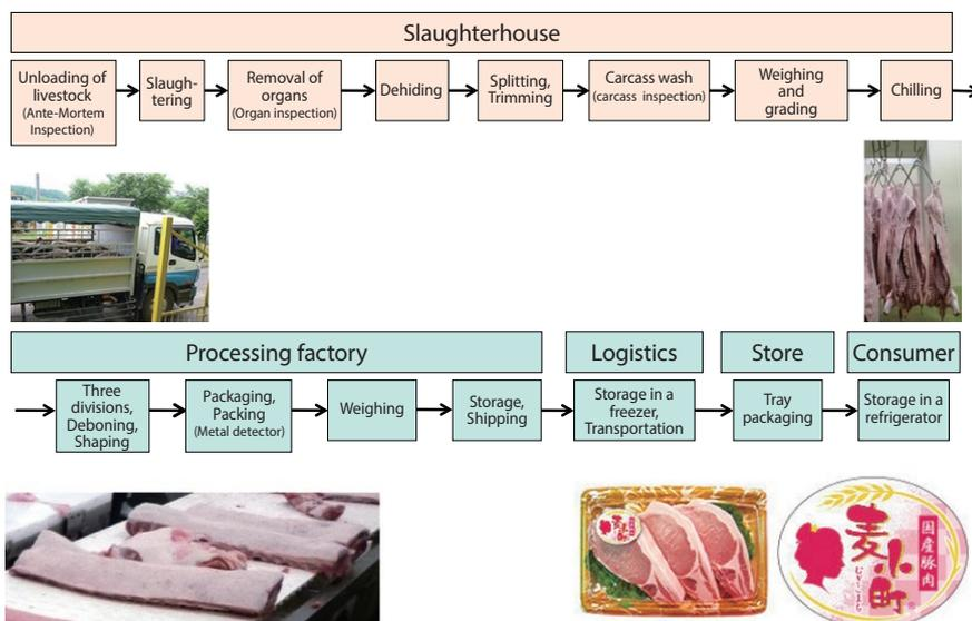
Figure 1: Production process in a pork processing factory
