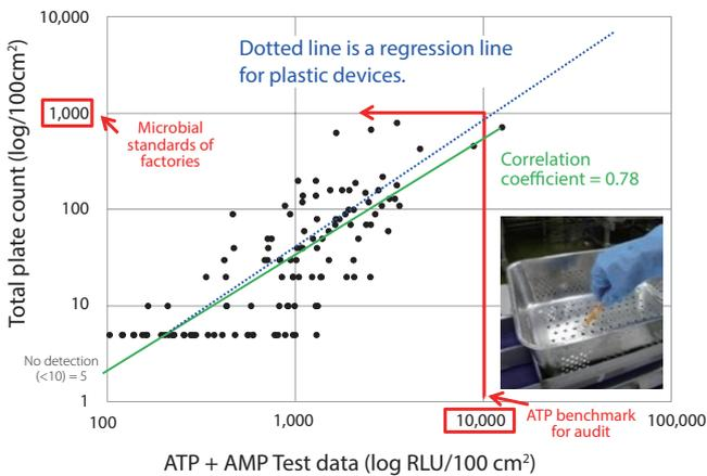
Figure 6: Correlation between an ATP Test and a microorganism test for metal equipment
