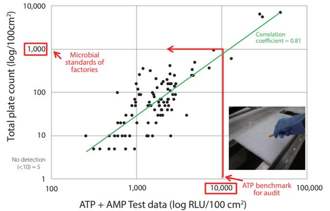
Figure 5: Correlation between an ATP Test and a microorganism test for plastic equipment
